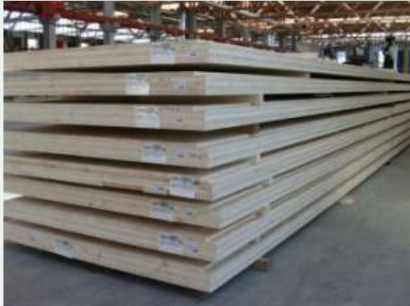
storage of CLT elements (production site)
